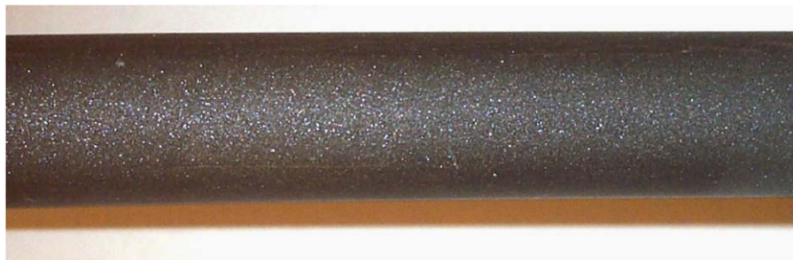
Fig. 1. An originally white corundum rod after exposure to hydrogen at 1400 °C.
